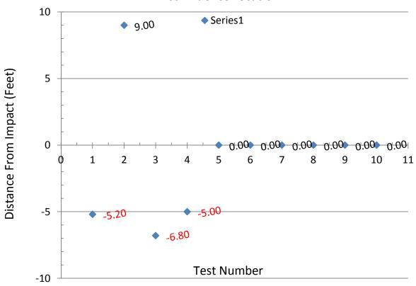
The above graph represents the location of the "1st" Evidence after impact. The longitudinal distance was measured from the impact location either forward or backward. In cases where the 1st Evidence lands before impact, the value is shown as a "RED" negative number.
